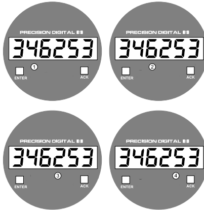
Figure 18. Display Showing Location of Set Point LEDs
