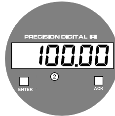
Meter displaying preset for set point 2
