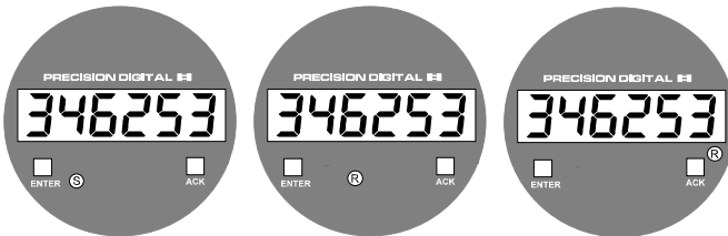
Figure 19. Display Showing Location of Set, Reset and Rate LEDs
